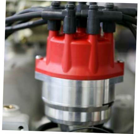
A high-performance distributor on one of Shelby and Roush's crate motors.
